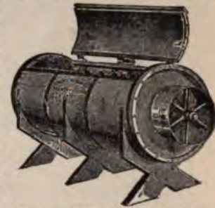
Fig. 199. Cylindrical factory churn.
